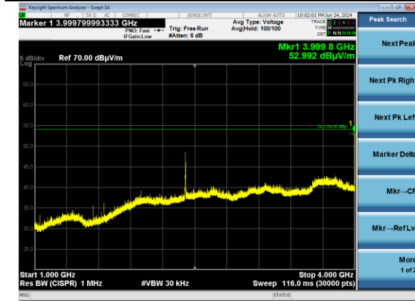
802.11a | Channel 157 | 6 Mbps | X Plane 1000-4000 MHz | Vertical
